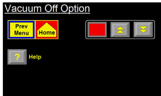
to apply the label, the Vacuum Valve will be turned off. The Vacuum Valve will remain off until the next Product Detect Input is received. This labeling sequence will require a slower product rate and a higher Label Placement amount so that the Applicator has enough time to completely dispense the label and activate the Tamp Valve. If the product rate is too high for the labeling sequence, the Product Rate Warning will be generated on the Display.
