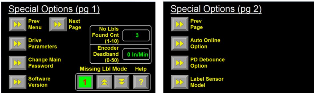
**Drive Parameters** - In this section, an operator can change the Accel/Decel rate of the motor and the maximum motor drive current setting
