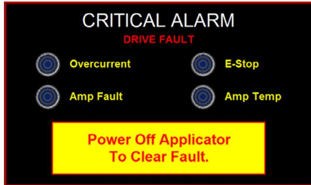
*Amp Fault* - If this occurs, there has been a failure on the Drive Board. The factory should be consulted if this occurs.
